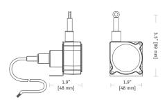
The SP3 from Celesco is a compact, economical stringpot that provides a user selectable 4-20 mA or 0-10 Vdc output signal. Simply install this sensor using the handy mounting bracket and connect the appropriate wires for the desired output.
