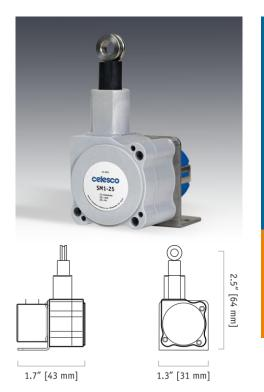
With its ultra-compact design the SM1 is the perfect solution when tight space is an issue. At just a little over an inch across, this miniature stringpot offers full stroke measurement ranges from 2½ to 25 inches. A precision plastic hybrid 10K-ohm potentiometer delivers a precise voltage divider output signal that is linearly proportional to the travel of the spring-loaded measuring cable.
