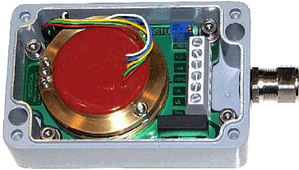
**Sensor box containing one highly sensitive servo inclinometer and one signal conditioner with  $\pm 5V$  output**
