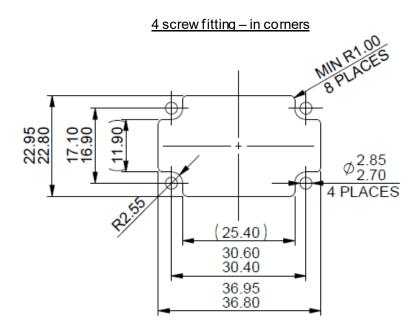
Curtiss Wright recommend the use of 4 x EJOT WN1451-K25-12 screws when utilising the 4 corner screw mounting points. The screws should be tightened to 0.3Nm with a minimum panel thickness of 3 mm. For thicker panels the screw length should be increased to suit.
