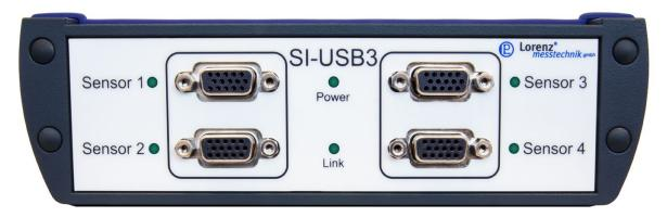
The four sensors are signed with Sensor 1 - 4. First the power supply must be connected. When a sensor is connected, the corresponding power LED is activated. Only when a PC/Laptop connection via the USB socket on the back exists, the Link-LED is activated. If the Link-LED is dark, check again the connection SI-USB3 to the PC/Laptop. Temperature measurements are possible at sensor connection 1 and/or sensor connection 4.
