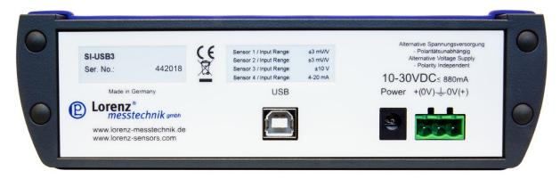
In addition to the serial number in the first field, the sensors and their associated connections are listed here in the second field.
