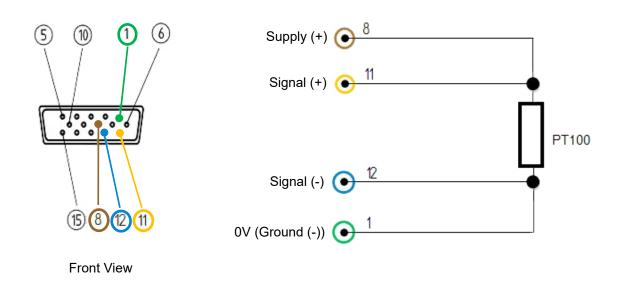
Connect the Signal (+) and Signal (-) wires as close as possible to the PT10
