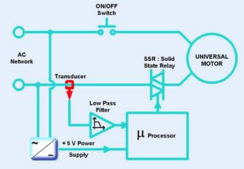
interesting to note the power supply sharing (+ 5 Volts) between the LTS or LTSR and the  $\mu$ processor.
