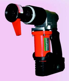
Indeed, the protection in an electrical torque wrench is the possibility to control the torque applied to tighten the screws. If an overtorque is applied to a fastener it can weaken or even rupture the fastener. If that bolt is used in the metallic construction of a high rise building or steel bridge where safety must be assurred 100%, the maximum torque in an electric torque wrench must be controlled.
